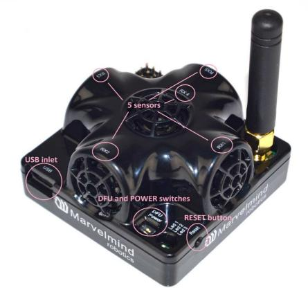
to press reset and modem is active. If modem is not active or works on different radio channel, the beacon automatically goes into a sleep mode in 1 minute
