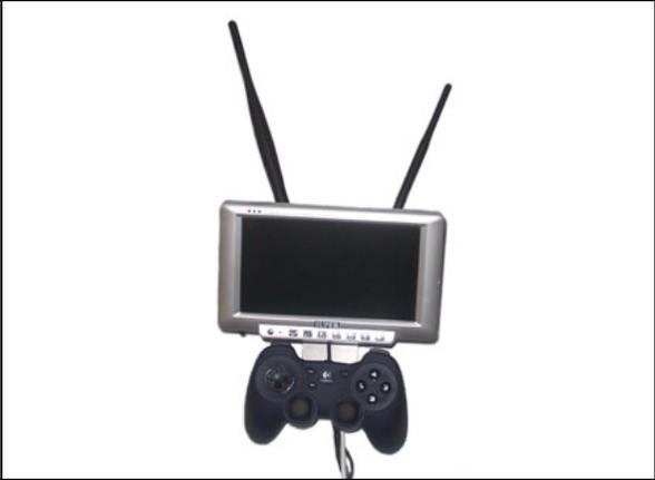
**WiFi Controller Option:** This option uses a WiFi connection similar to the one above, but utilizes a Ultra-Compact PC. The Color touch screen LCD can be used to control the robot and view the IP camera(s). The PC is mounted in a custom bracket with a gamepad controller mounted to it. We provide a program so all the driving and control of the robot is done using the using the robot control program using the game pad controller and touch screen LCD.
