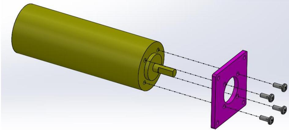
2. Use the included #4-40 hardware and plastic spacers to mount the motor plate to the motor tube.
