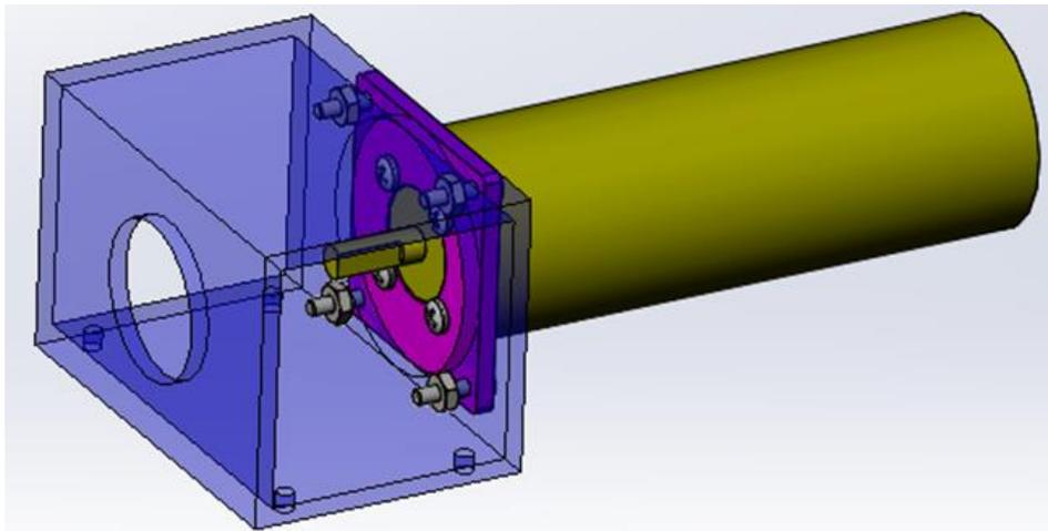
3. Mount motor tube to chassis with provided hardware, (1/4-20 Screws/Nuts), using Loctite or locknuts.
