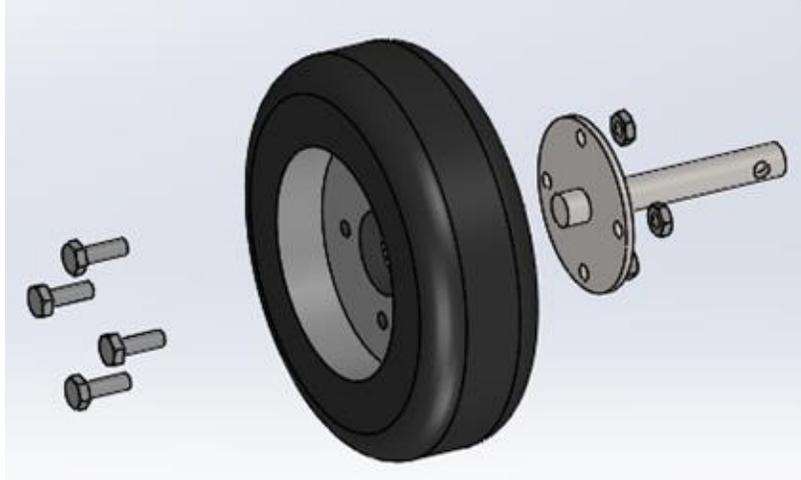
6. Mount wheel assembly to motor assembly. Slide a lock collar over the shaft before installation. Insert wheel shaft through ball bearing. Before sliding the wheel shaft onto the motor, slide on a second lock collar. Align the set screw holes on the wheel shaft and the lock collar to the flat spot on the motor shaft. Firmly press the wheel shaft inward against the motor and secure the set screw with Loctite.
