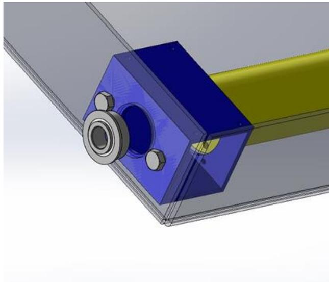
5. Mount wheel to wheel shaft. Ensure air is let from tire until it is soft and easy to work with. Avoid pinching the inner tube when mounting. Use Loctite, locknuts, or jam nuts to secure the wheel to the shaft. Air up the tire according to the specifications on the side wall of the tire.
