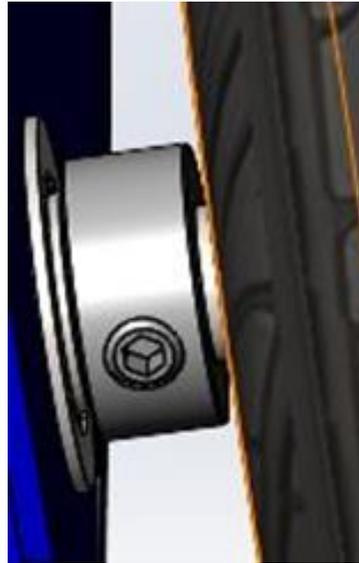
8. Install standoffs onto main chassis with provided hardware. Use Loctite to secure screw to standoff on the chassis.
