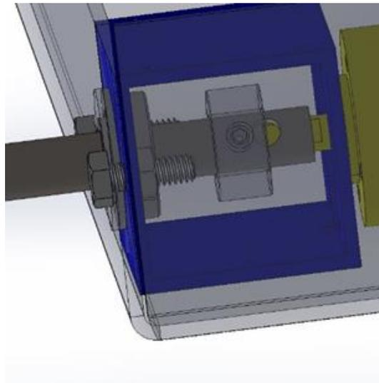
7. Slide the first lock collar up against the ball bearing on the outside of the chassis and secure with Loctite. This will keep the ball bearing from sliding out away from the chassis.
