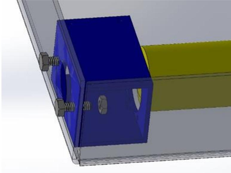
4. Insert ball bearing to support the wheel shaft. Additional filling may be needed to fit bearing through chassis into motor tube. Test fit each bearing to find the bearing that works best for each bearing hole.
